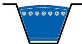
Belt wear rough grooves, slip, overload
